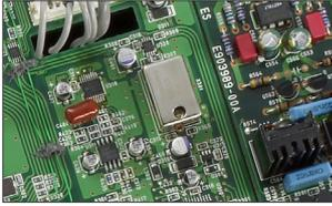
A newly designed high-precision clock is implemented to achieve the highest level of sound quality for an all-in-one digital player. A VCXO (voltage controlled crystal oscillator) of  $\pm 0.5$  ppm (\*2) that uses a large crystal is deployed in the K-01, which is
