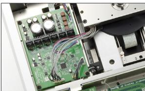
The driver circuit of the transport mechanism was newly designed specifically for audio playback, to accomplish smoother and higher-accuracy servo control. The VS-DD (VRDS Spindle Discrete Driver), a newly designed discrete amplifier circuit,
